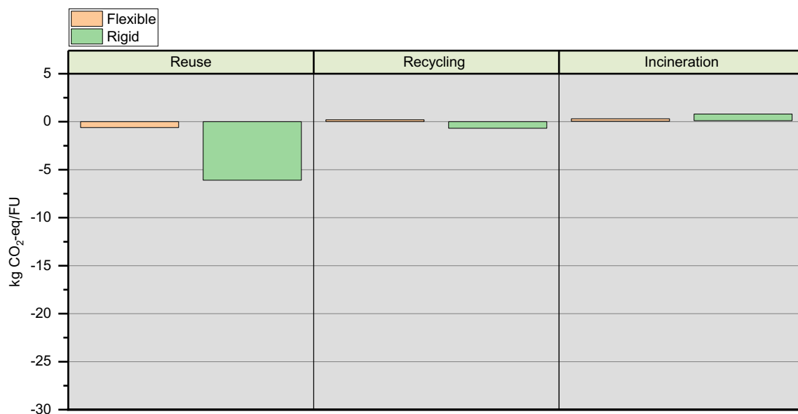
Figure 7 - Potential environmental impacts within climate change related to the production and end-of-life management of rigid and flexible packaging products made of PE. The result intervals represent a 95% confidence interval and are presented as kg CO 2 equivalent per functional unit (FU).
