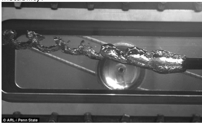
Figur 2 Photograph of a second order pulsating supercavity in the Penn State ARL Garfield Thomas Water Tunnel facility's 12-inch diameter water tunnel. The circular object is a window mounted hydrophone.
