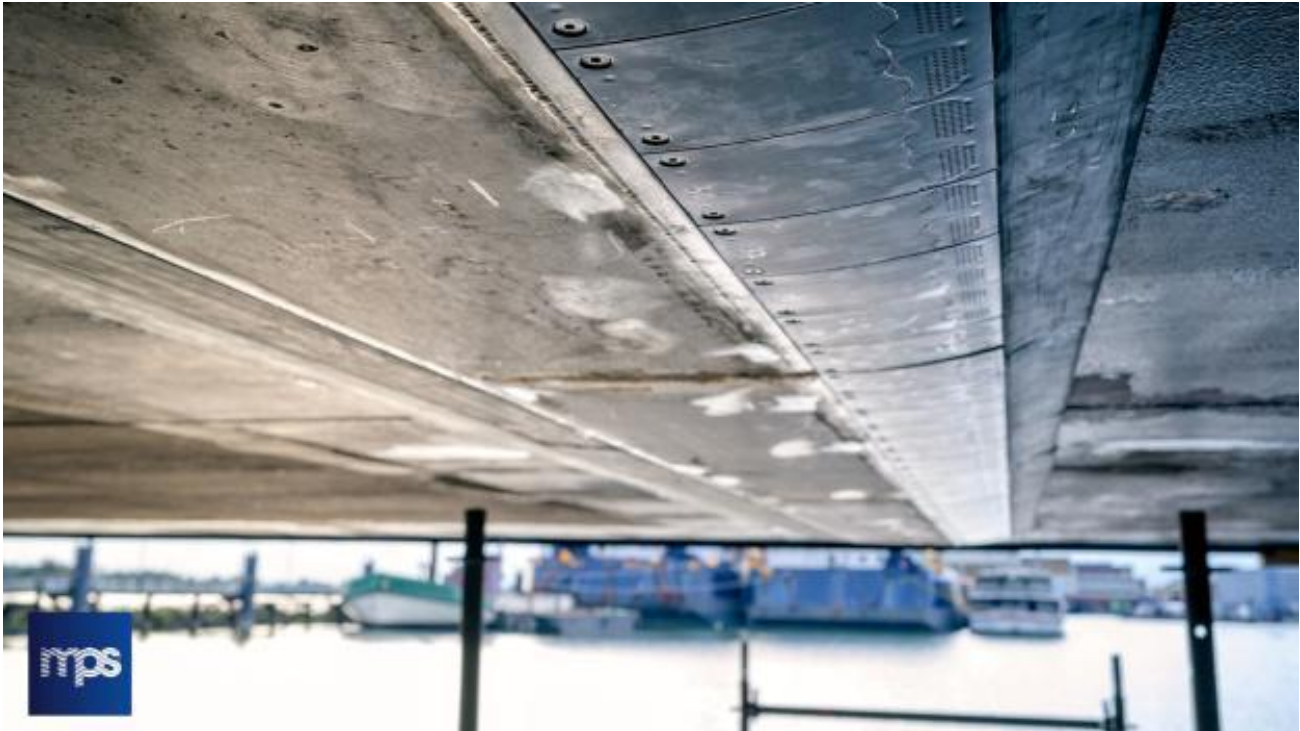
An example of one of the bands with fluidic oscillators that create about 240,000 micro-bubbles per second per metre along the ship's hull. Illustration: Marine Performance Systems.
