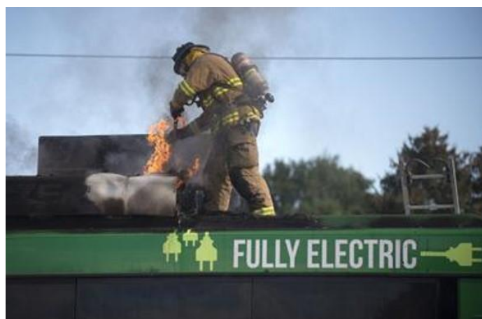
Figure 12. A firefighter was suppressing the fire of the faulted battery on the top of the electric bus [114].
