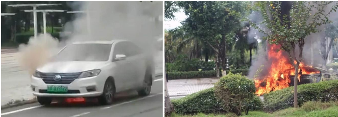
Figure 8. The fire scene of a Lifan 650 EV, where the fire started at the battery pack installed in the vehicle chassis, and EV was completely destroyed by fire without effective fire suppression [108].
