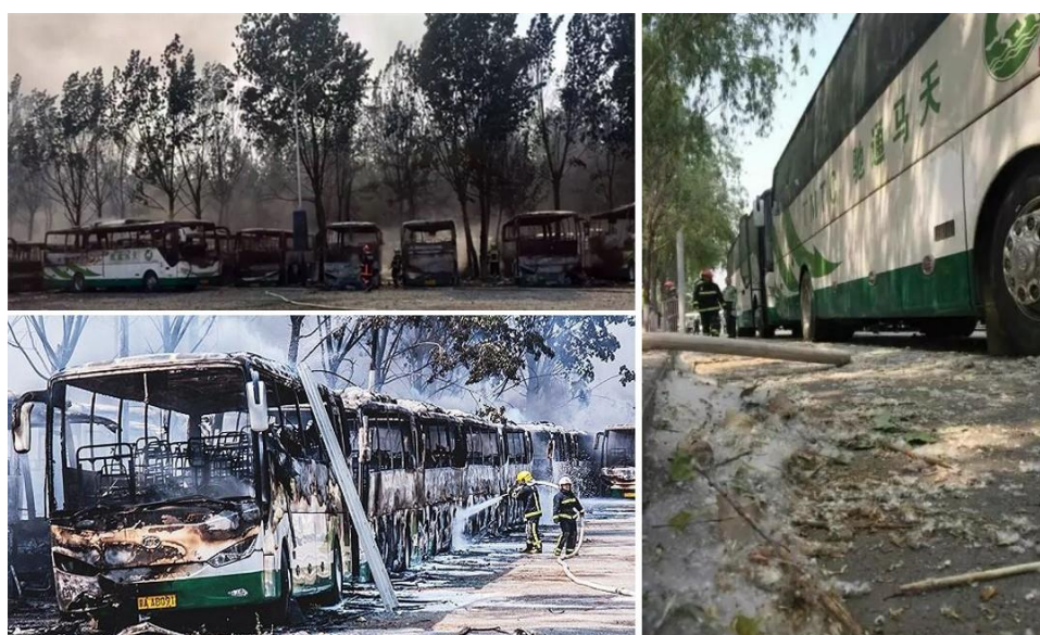
Figure 13. A chain fire on electric buses in Beijing, China in 2017, where firefighters used an extra amount of water to cool down buses to prevent the battery reignition, and piles of catkins was considered as the initial fire source [115].
