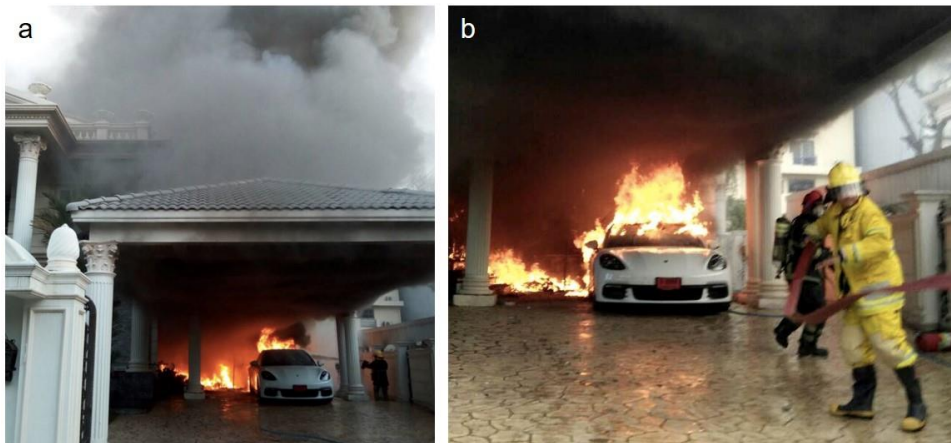
Figure 17. The PHEV Porsche Panamera got on fire during charging on 16 March 2018 Thailand:(a) the fire was intense and damaged the owner's house; (b) firefighters tried to extinguish the fire using water [126].
