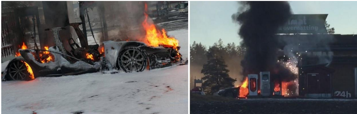
Figure 10. The fire on a Tesla Model S while being charged at the supercharging station in Norway on 1 January 2016, where the fire also spread to the passenger compartment [110].
