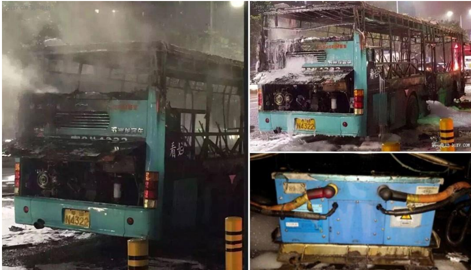
Figure 15. The hybrid-electric bus fire accident on 16 March 2016 in Shenzhen, China, where the battery box is intact after fire [124].
