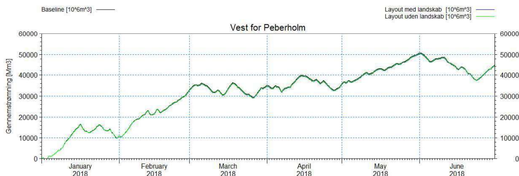
Figure 6-126 Cross-sectional flow west of Peberholm with the existing conditions (black curve) reclamation without landscape (green curve) and reclamation with landscape (blue curve).
