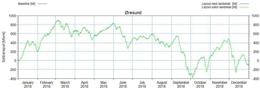
Figure 6-147 Accumulated transport of salt in the cross-section east of Peberholm with the existing conditions (black curve), reclamation without landscape (green curve) and reclamation with landscape (blue curve).
