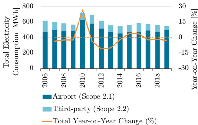
Figure 13. Total annual electricity consumption and year-on-year change (%) from 2006 to 2019. Source: Energi Danmark (2020); Midtjyllands Airport (2020).
