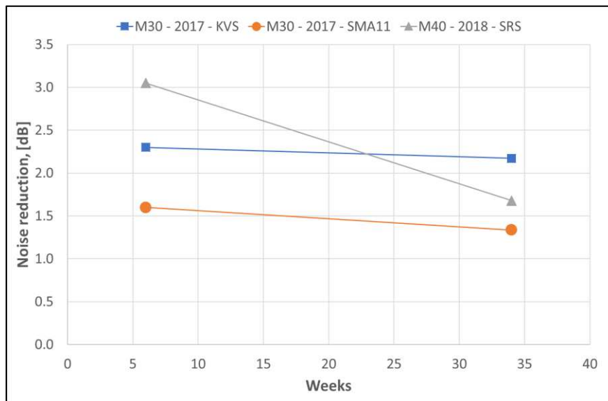
Figure 21 – Noise development from week 6 to week 34, KVS (M30-2017), SMA11 (M30-2017), SRS (M40-2017)
