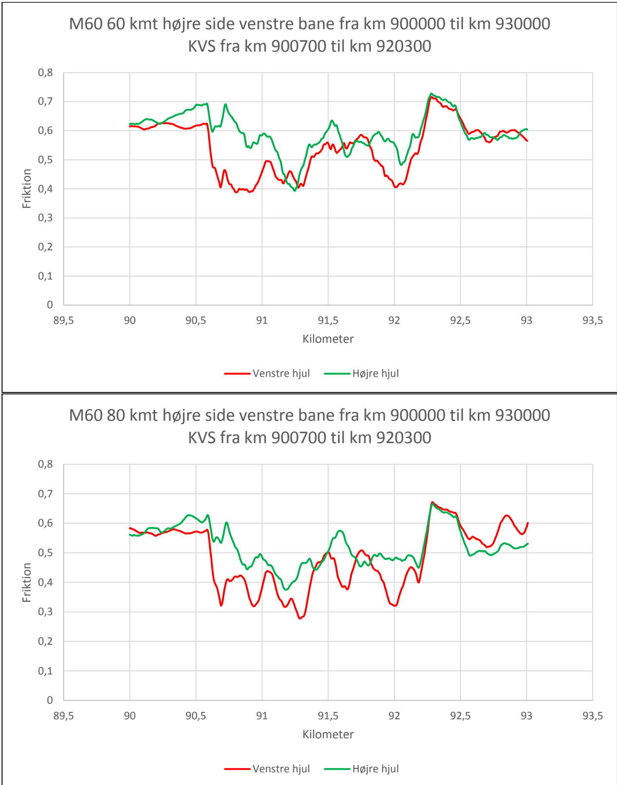
Figure 16 – Friction on M60, right side and left lane at 60 (top) and 80 km/h (bottom).
