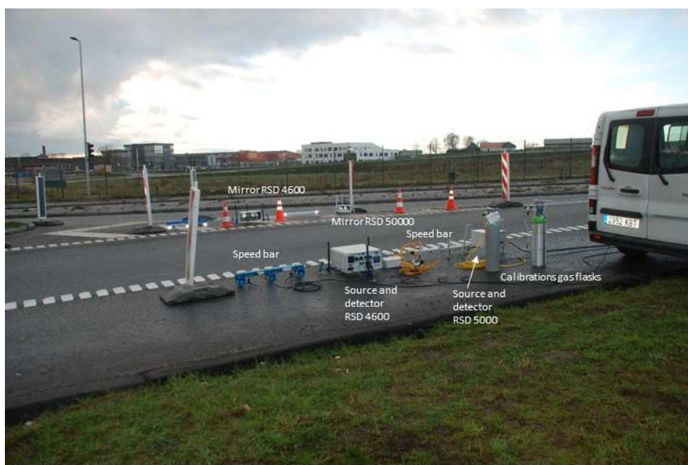
FIGURE 2.1. The setup for the remote sensing measurements with parallel measurements using RSD 4600 and RSD 5000. The measured heavy-duty vehicles passes between the Source and detector units and the mirror units. As can be seen there are about 1.5 m between the two instruments and the instruments are therefore not measuring on the exact same exhaust from the heavy-duty vehicle. Two cameras, one for each instrument, are placed about 10 m further up the road in order to take pictures of the heavy-duty vehicles from the front. There are also two set of speed bars, one for each instrument, that measures velocity and acceleration as close as possible to the emission measurements. The computers controlling and storing the measurement results are placed in the white van. The photo is taken at the measurement site in Køge.
