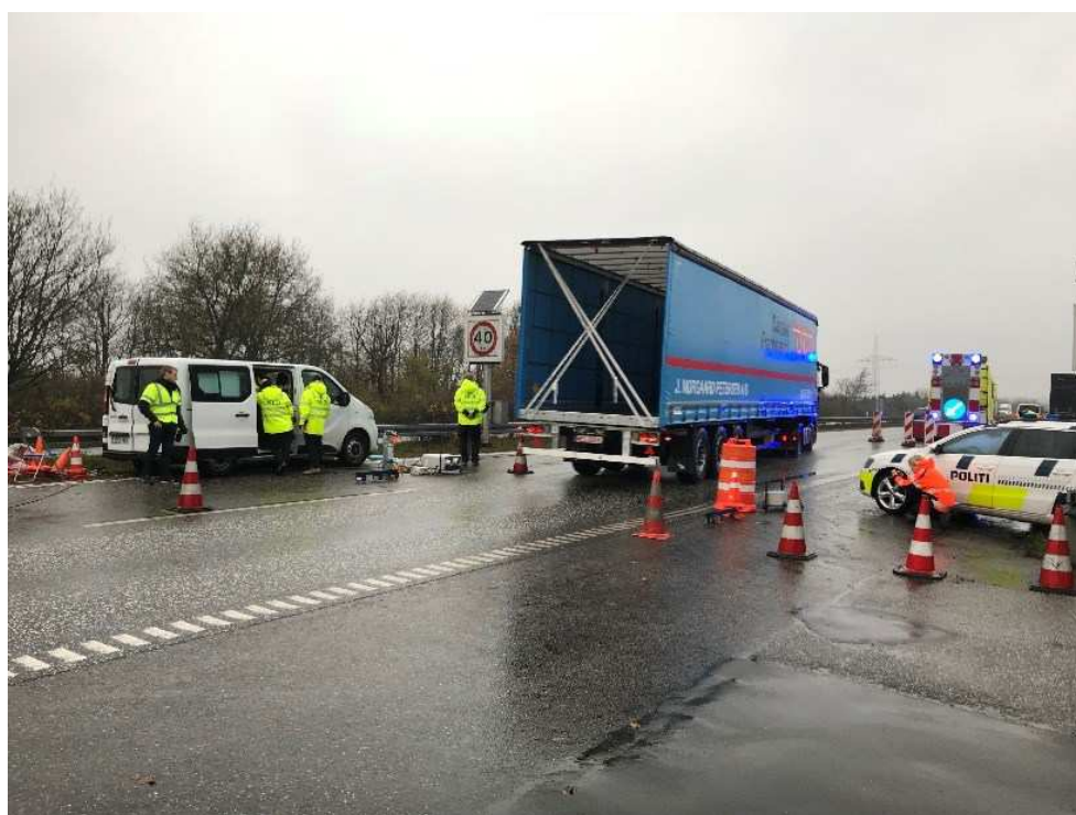
FIGURE 2.5. Measurements at the Danish Polices control area at the Danish-German Border in Padborg on road E45 north bound. The source and detector unit is placed close to the white van at the left site of the road. The mirror is placed opposite at the right site of the road. The setup with the warning vehicle and warning signs is part of the Danish Polices normal arrangements for control of the vehicles passing the border
