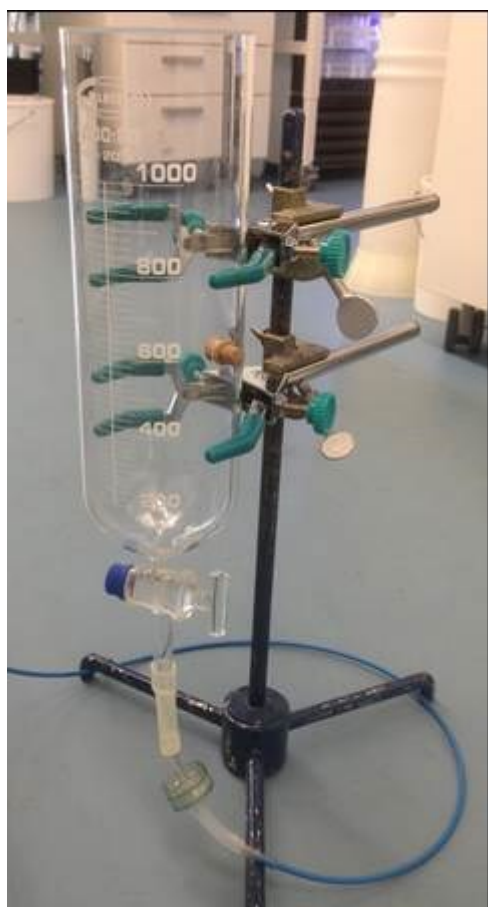
Figure 20. Gravimetric separation funnel. The blue line supplied the compressed air (CA) for aeration. Between the tubing connecting the glass funnel to the CA, an air filter was placed to reduce contamination. At the 600 mL mark there was a side port with a cork stop, to allow for draining the fluid containing low density particles
