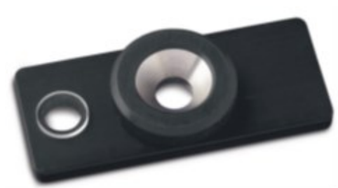
Figure 23. Compression cell for transmission mode imaging. The cell is only used for evaporating the sample onto a well-defined area of the transmission window, and, despite of its name, never actually used to compress two windows.
