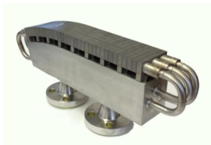
Prototypes of the Elements of the First-Wall Blanket Modules (above) and Divertor (below), the latter after testing at high heat fluxes (Photos courtesy of Atmosstat and Ansaldo Nucleare)
