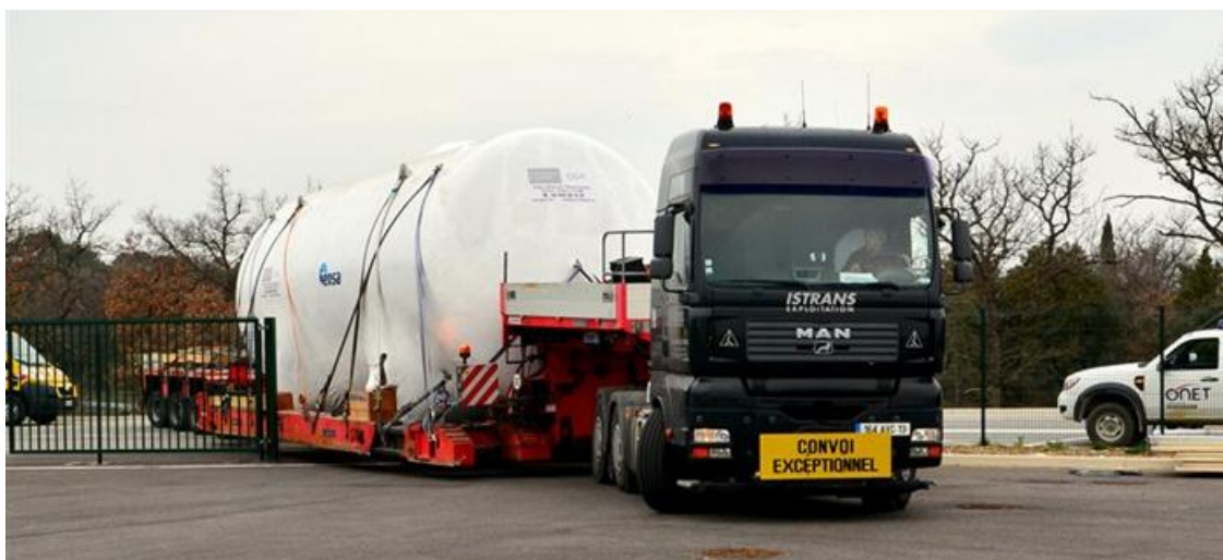
Delivery of a 100 m 3 WDS tank to the ITER Organization – among the first European deliveries
