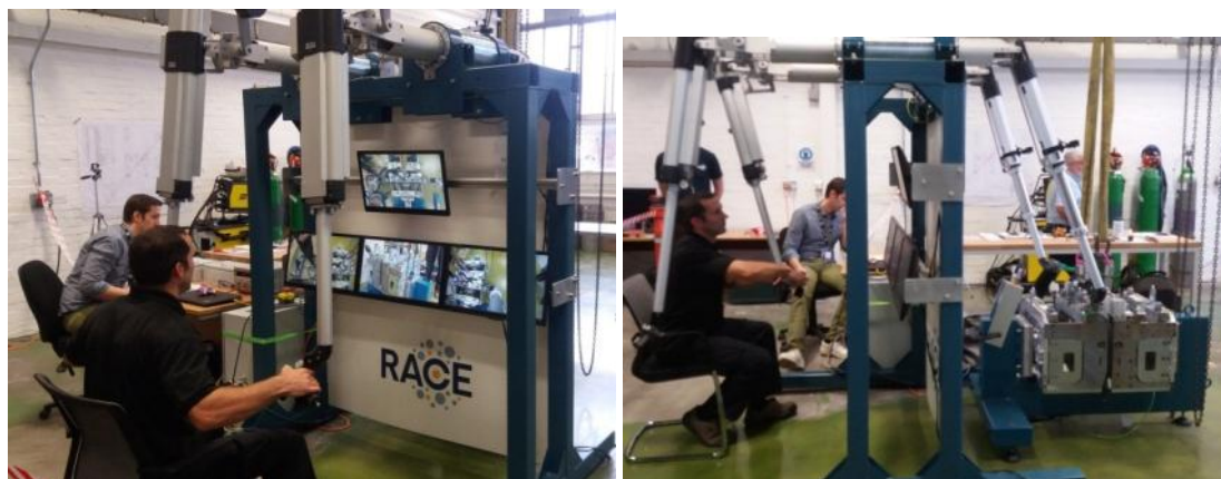
Photos showing the simulated Remote Handling conditions for operating the tooling for cutting and welding the cooling pipes of the Neutral Beam components
