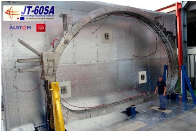
A superconducting Toroidal Field Coil (one out of the 18 to be provided by the EU) at the factory
