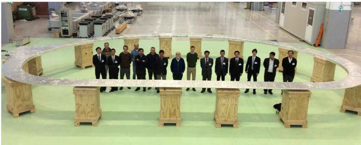
First full size Double Pancake prototype for the Toroidal Field (TF) Coils showing the scale of the superconducting coils which are some of the largest ever produced
