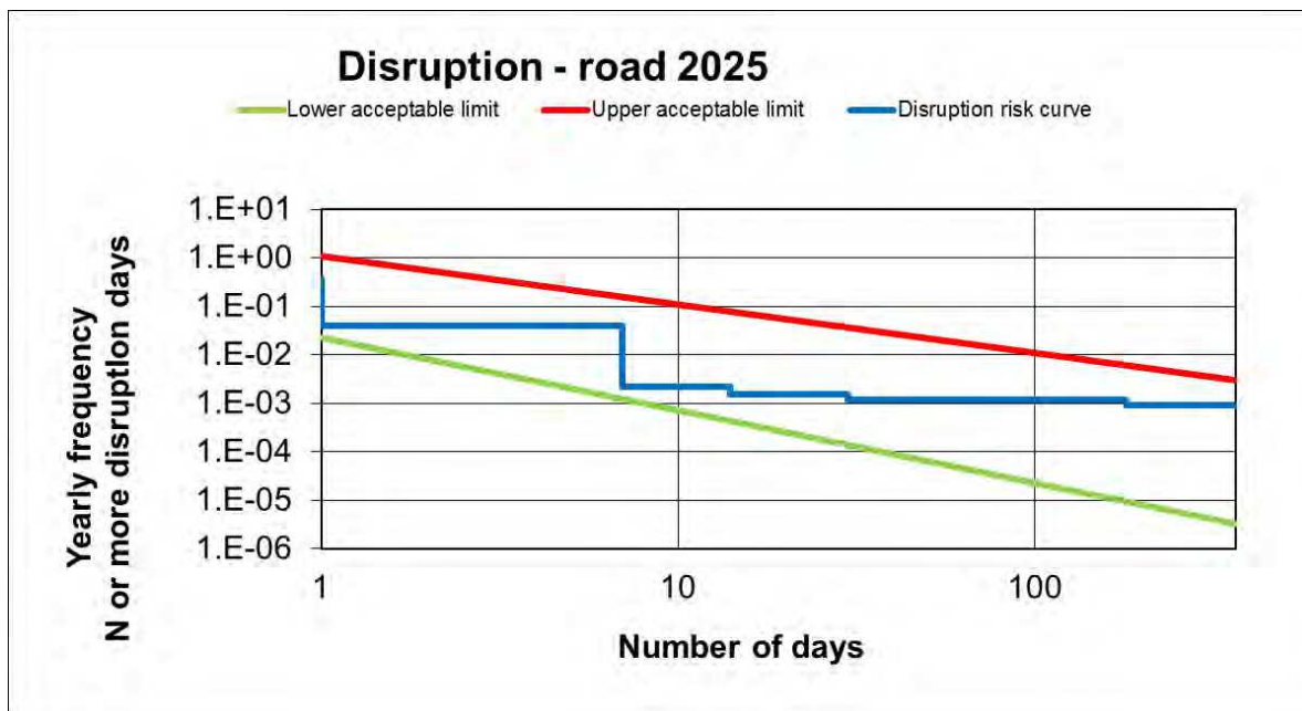
Figure 6-1 FN-curve for the disruption of the road part (one tube only) (2025)
