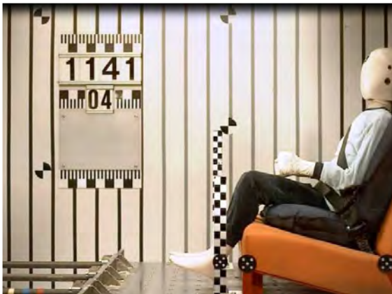
Figure 2a: Time 0 ms – Initial P10 dummy position
