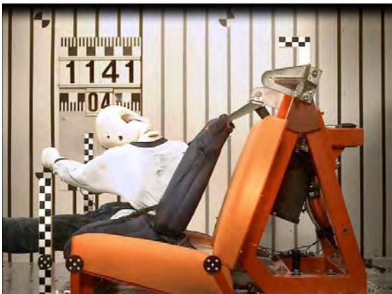
Figure 2c: Time 80 ms – Start of the submarining – The lap belt has intruded into the abdomen.
