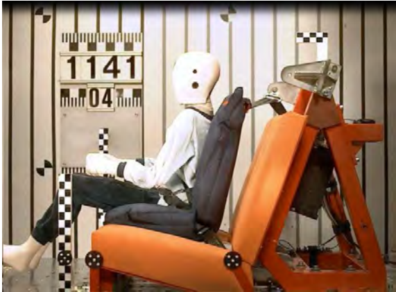
Figure 2b: Time 40 ms – P10 dummy and belt geometry during loading phase
