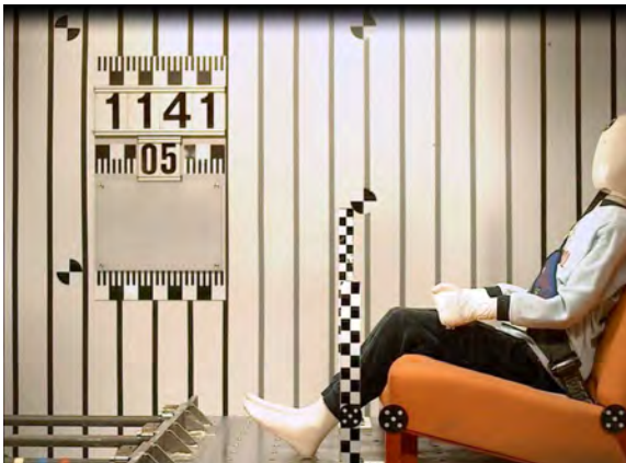
Figure 2a: Time 0 ms – Initial P10 dummy position
