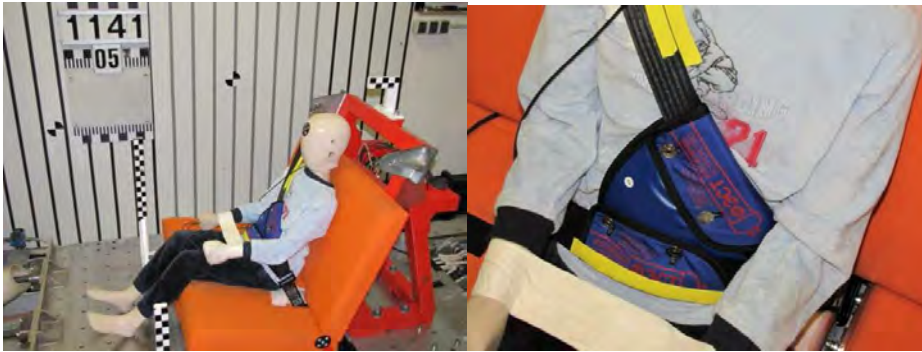
Figure 1: test set-up with belt guide device using the P10 dummy
