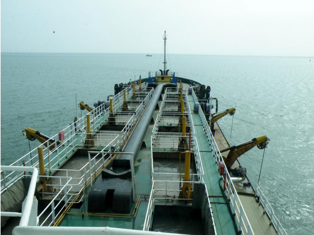
The dredger has bottom doors facilities 12 units.
