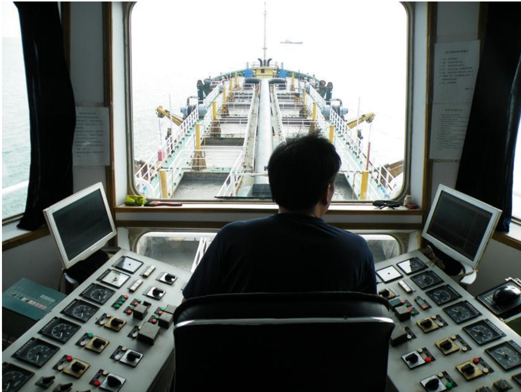
The dredger has two suction tubes operated of 1 person from the bridge
