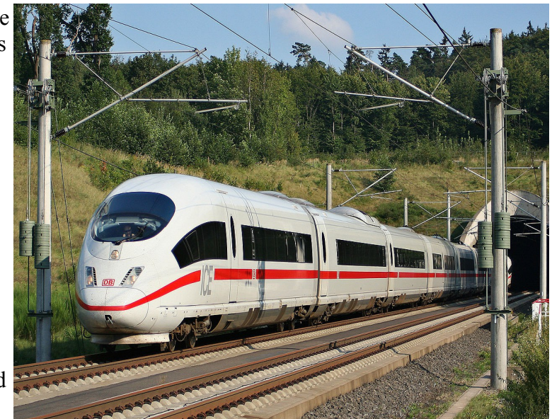
Picture 9: Image source - Wikimedia commons. ICE3, Siemens Valaro family. With a top speed on paper at between 320 and 380km/h, so the speed is limited mostly to 250 to 300km/h
