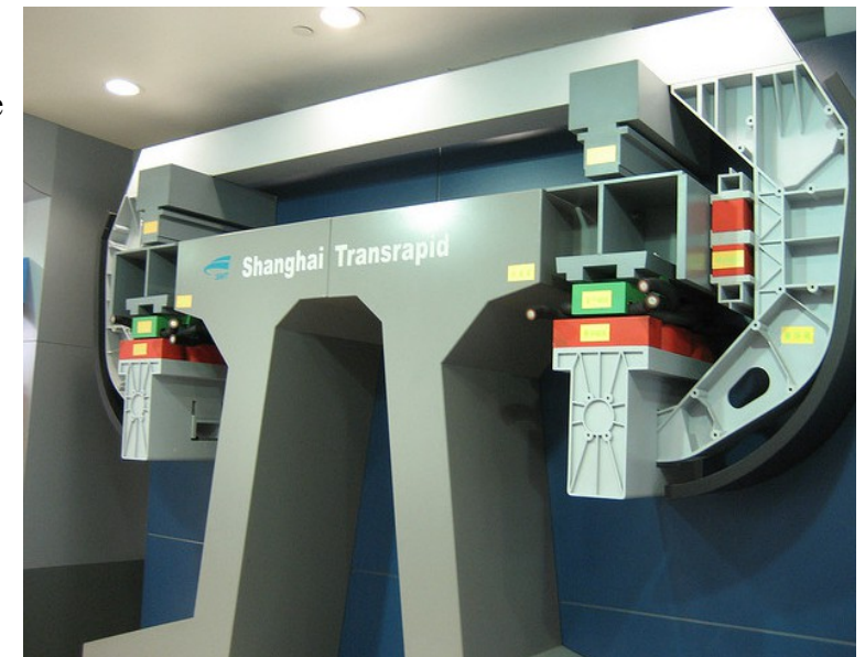
Picture 6: Image Source - SMT. Picture depicts section of a TR08 system.
