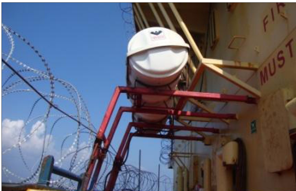
Figure 10: Picture of the liferafts on the starboard side on the LEOPARD. Source: Private photo.
