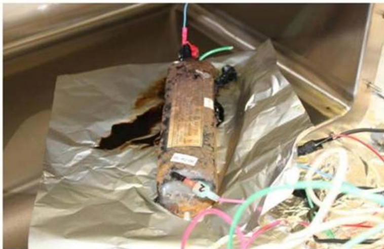
Figure E.7. The light ballast that burst during the emission test with electrical load
