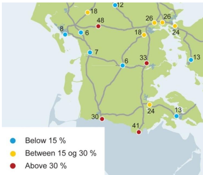
Map 3.1.1 Increase in traffic (in percentage) at selected sites in the southern part of Jutland, 2000 – 2010.
