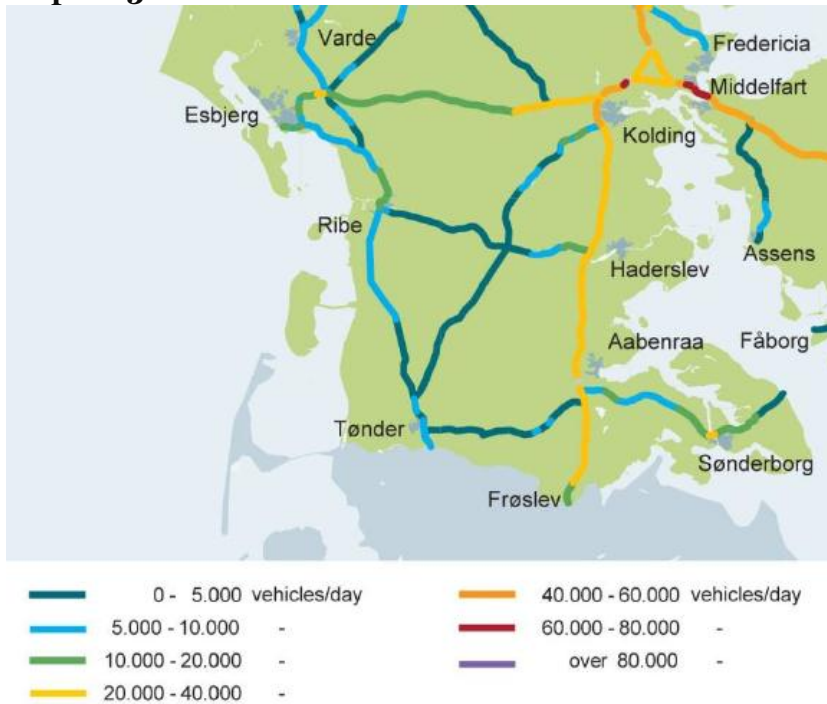
Map 2.1.3 Number of vehicles on the trunk roads in the southern part of Jutland (2011)
