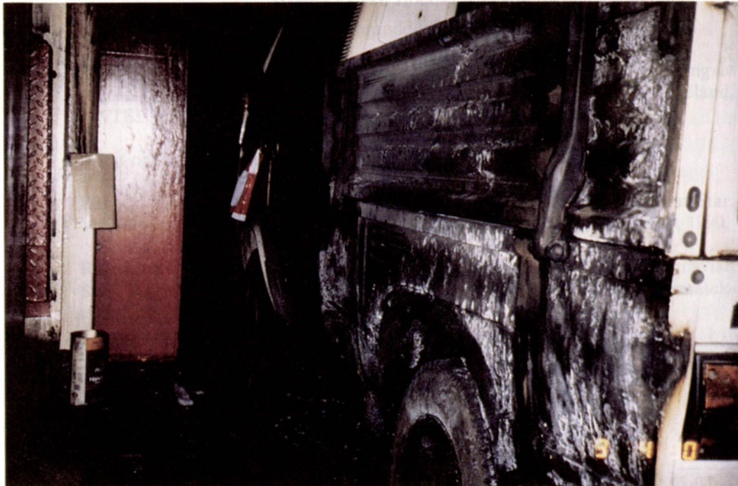
Figure 11. Photograph showing a car damaged by fire. The car was parked just nearby the open sliding door no. 9 (A 60), see Figure 3, on the car deck. The air velocity trough this specific fire door opening has been measured to 20 m/s (during a full scale test on board a sister vessel) without the thermal effects from a fire. Note that this velocity refers to cold air. At a smoke temperature of 600°C the velocity increases by approximately a factor 3. This indicates the large effect that the ventilation system would have on the main fire.
