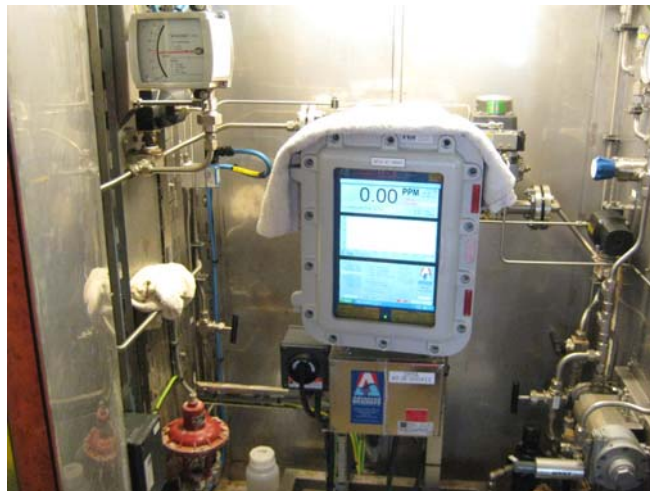
Figure A4.4 Continuous OiW Monitoring System EX1000 (Advanced Sensors), Dan FF
