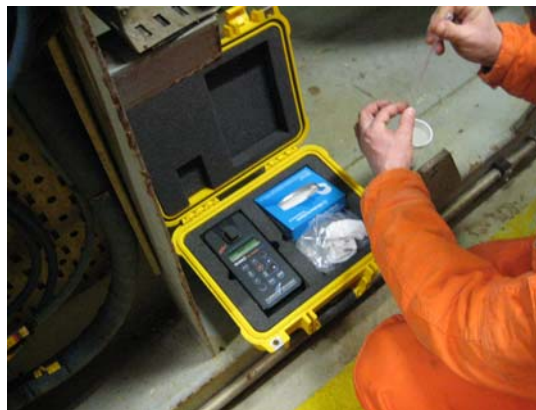
Figure A5.4 Quick Analysis of Skjold OiW using Turner TD5000
