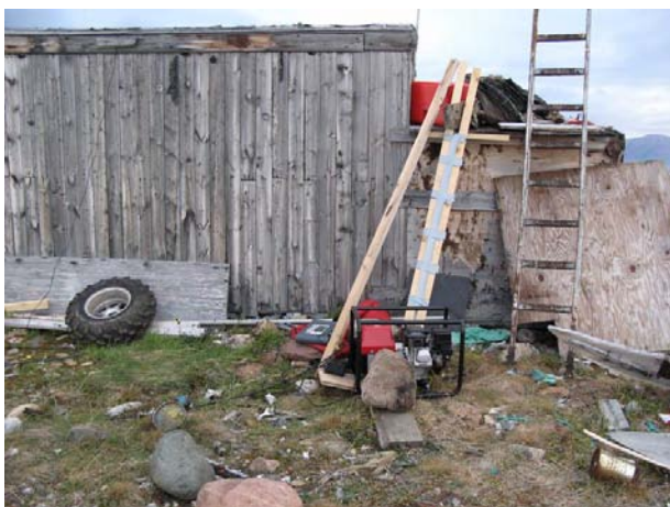
Figure 4. Generator used for the air sampler. Tubing from fuel tank on roof to generator protected from direct sunlight to avoid gas formation.
