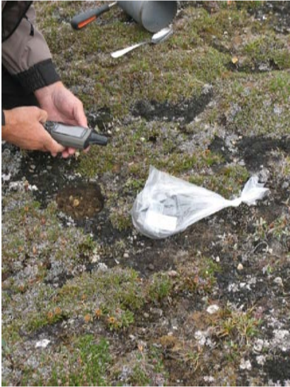
Figure 9. Sampling of soil and recording of GPS coordinates.
