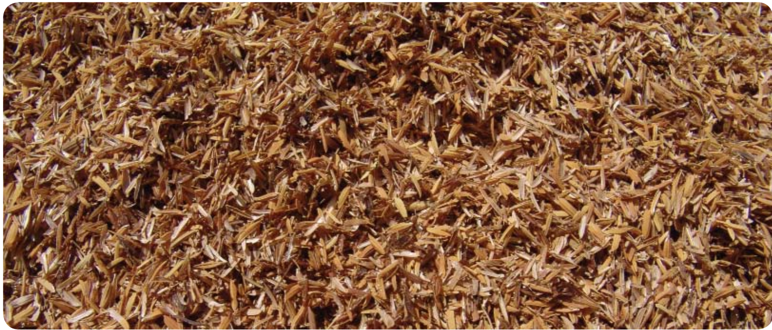
The plant at Bua Yai consumes 220 tonnes of rice husks a day, and the electricity produced displaces electricity based on fossil fuels.
