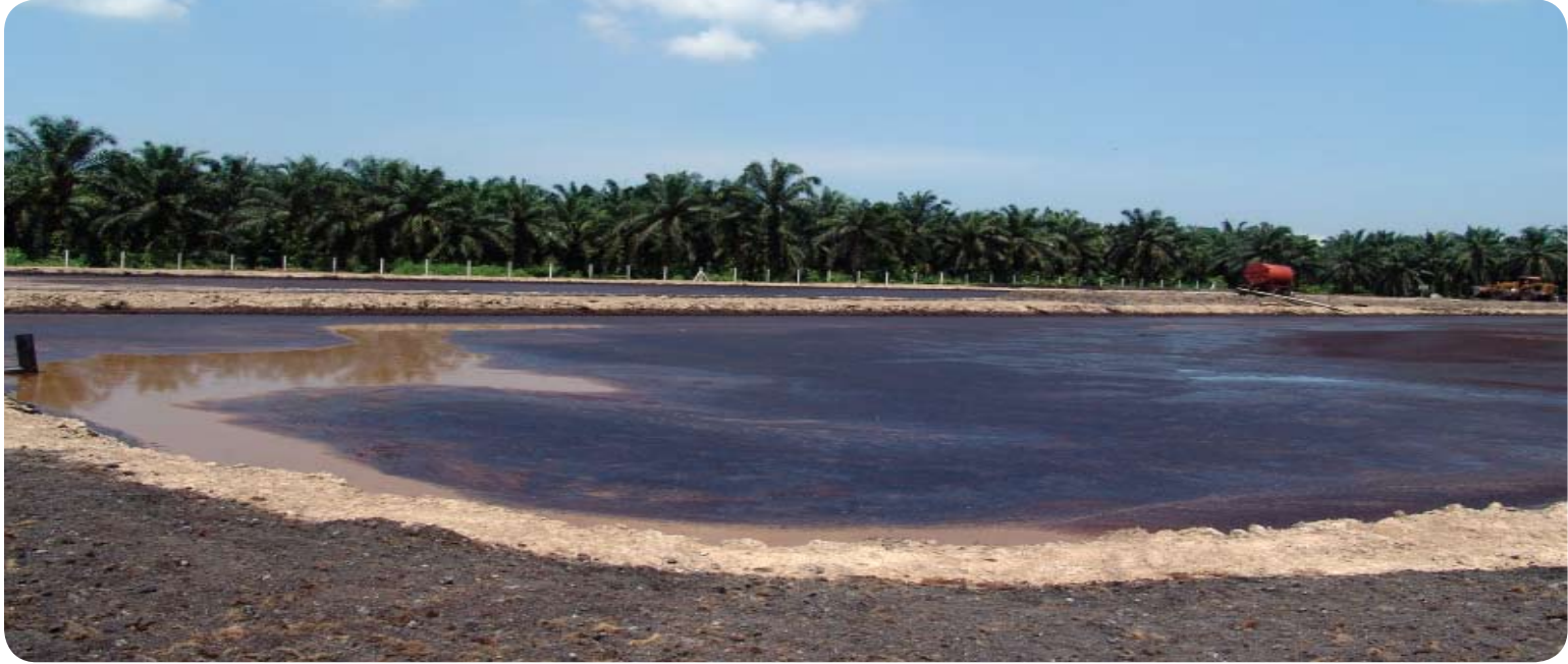
The open lagoons, with decomposing residues are emitting methane into the atmosphere. The new cdm project will reduce emissions and produce high quality organic fertilizers instead.
