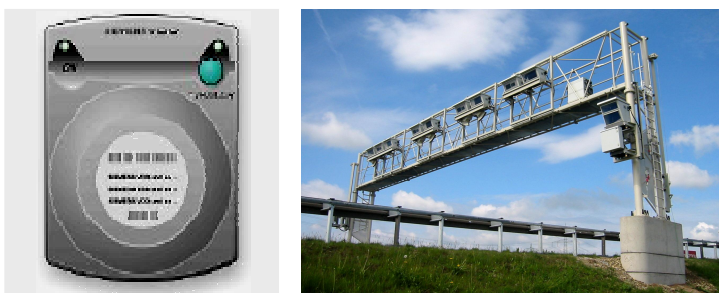
Figure 3: GNSS/CN OBU: possible solution of a thin client and a German enforcement station using IR beacons
