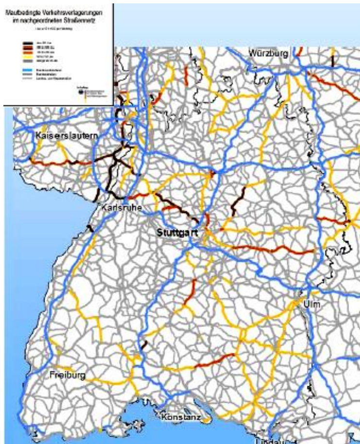
Figure 19: Detour Traffic in SW-Germany after implementation of LKW-Maut (dark segments show HGV increase)
