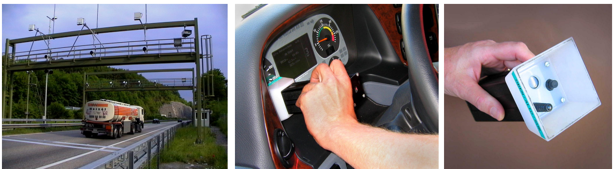
Figure 10: LSVA enforcement station and tachograph camera to check the mileage of vehicles without OBU
