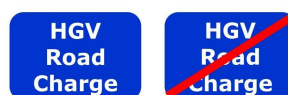
Figure 18 : Fictitious road traffic signs for marking where the user enters and exits the obligation to pay. Existing charging schemes feature no such signs, since small adaptations to motorway signage (for network charging) or to border crossing signage (for area charging) are sufficient to communicate the obligation to pay.
