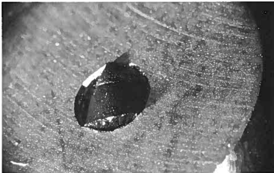
Figure 9: Missing piece of O-ring in Figure 8 still residing in orifice hole.
