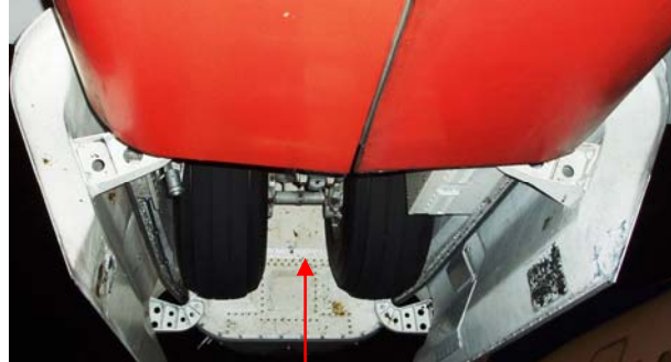
MLG position in the right MLG wheel well
