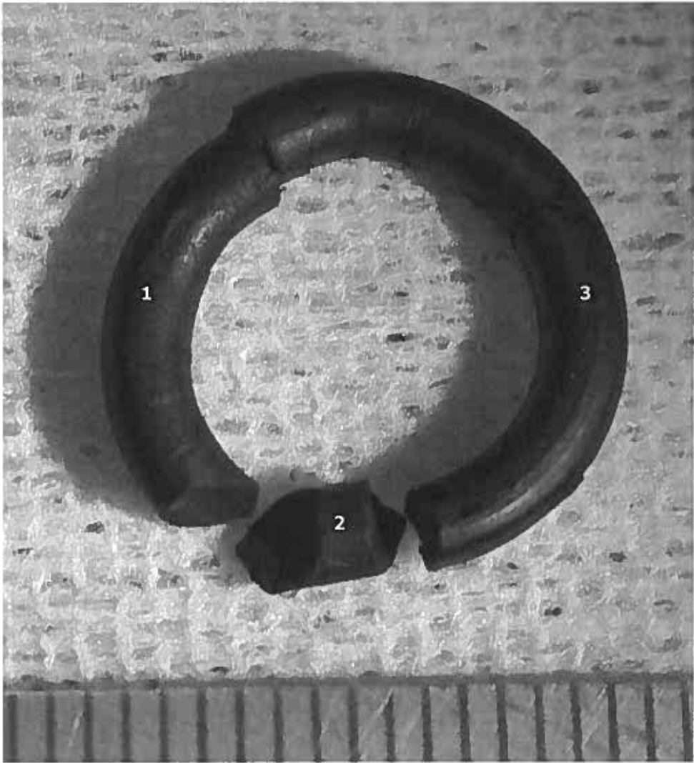
Figure 7: Retrieved parts of O-ring material trapped between cone and housing.
