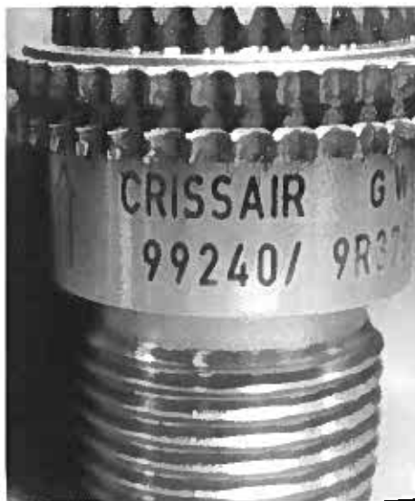
Figure 1: External views of the blocked flow restrictor (labelled SN 074).
