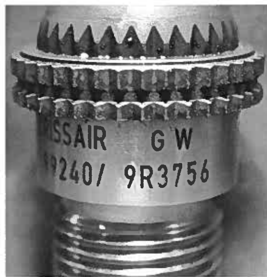
Figure 1: External views of the blocked flow restrictor (labelled SN 074).
