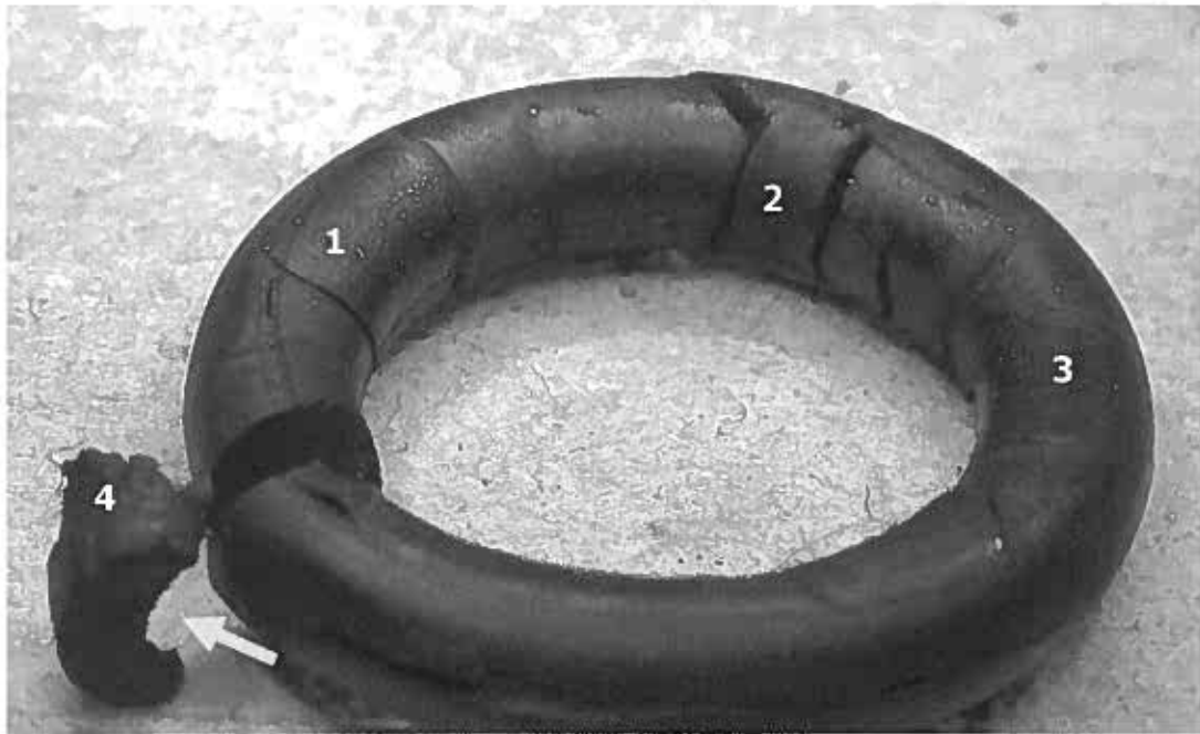
Figure 8: Reassemble of O-ring using all retrieved material except the small piece still residing in orifice hole. The arrow points to where the missing piece fits.
