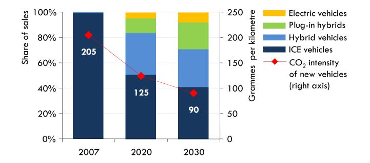
Improvements to the internal combustion engine & the uptake of next-generation vehicles & biofuels lead to a 56% reduction in new-car emission intensity by 2030
