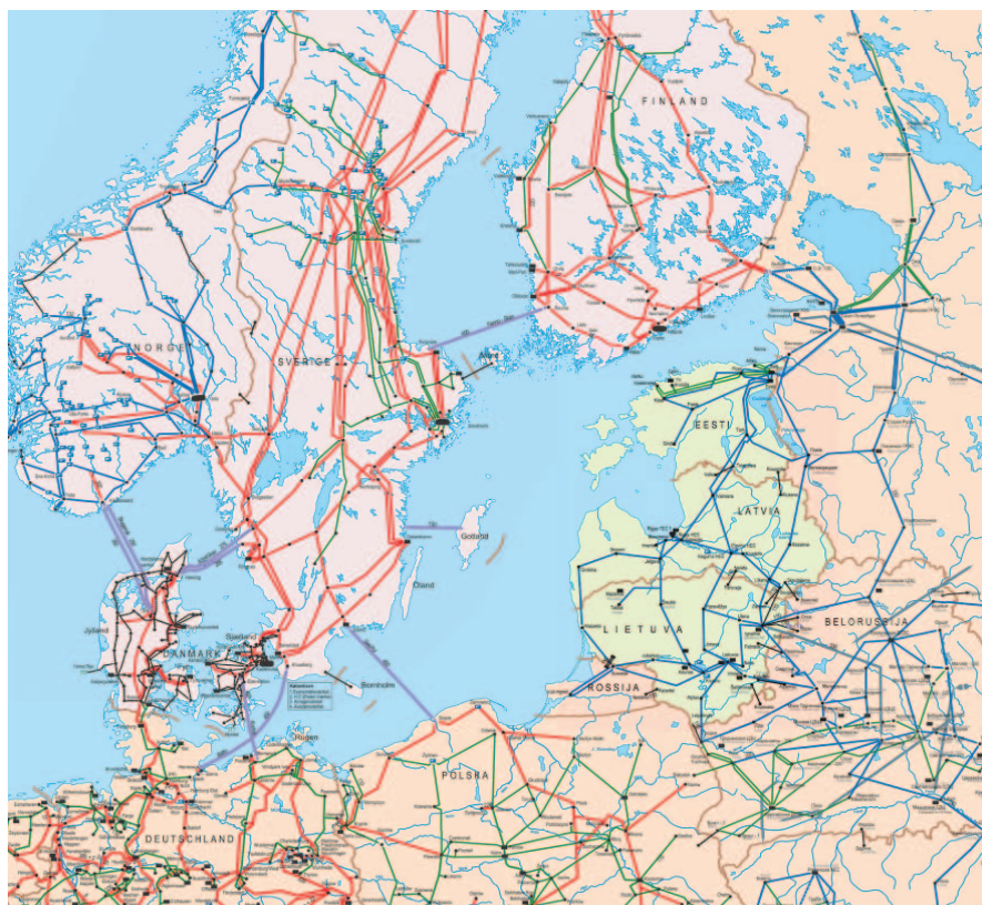
Figure 17: Map of the transmissions grid in the Baltic Sea Region (Source: Nordel)
