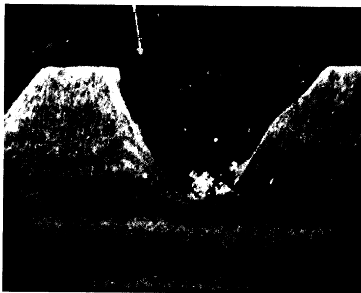
Figure 22: Minute crack in thread bottom.
