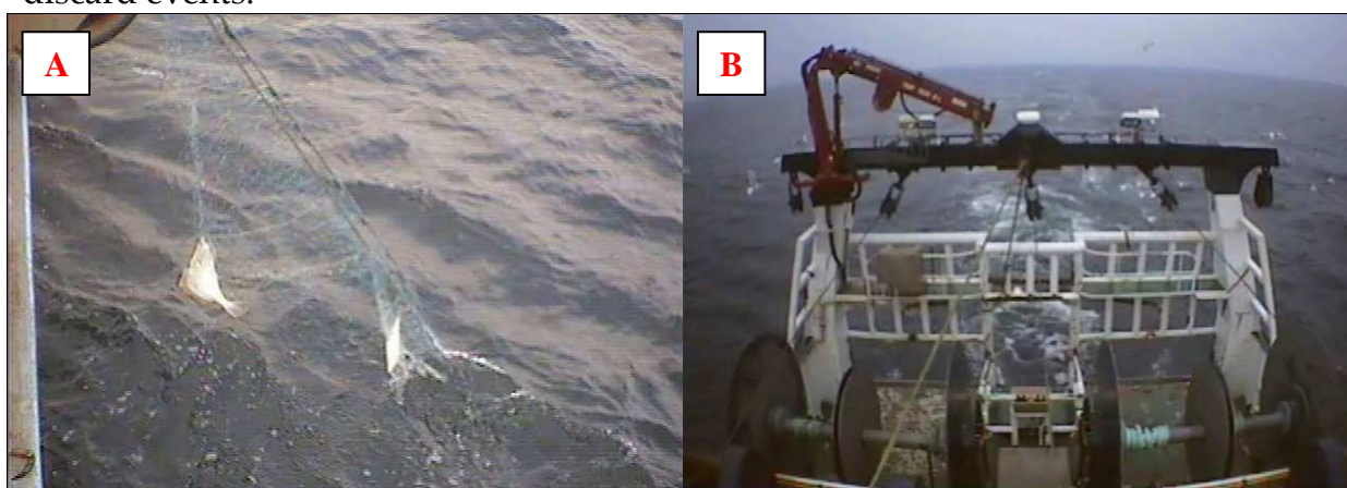
Figure 12. Example images from two of the participating vessels for monitoring the net coming on deck in order to assess for any discarding of catch. Image A-good view of net coming on deck to assess for discards. Image B-Poor view for seeing the net coming on the stern of the deck.
