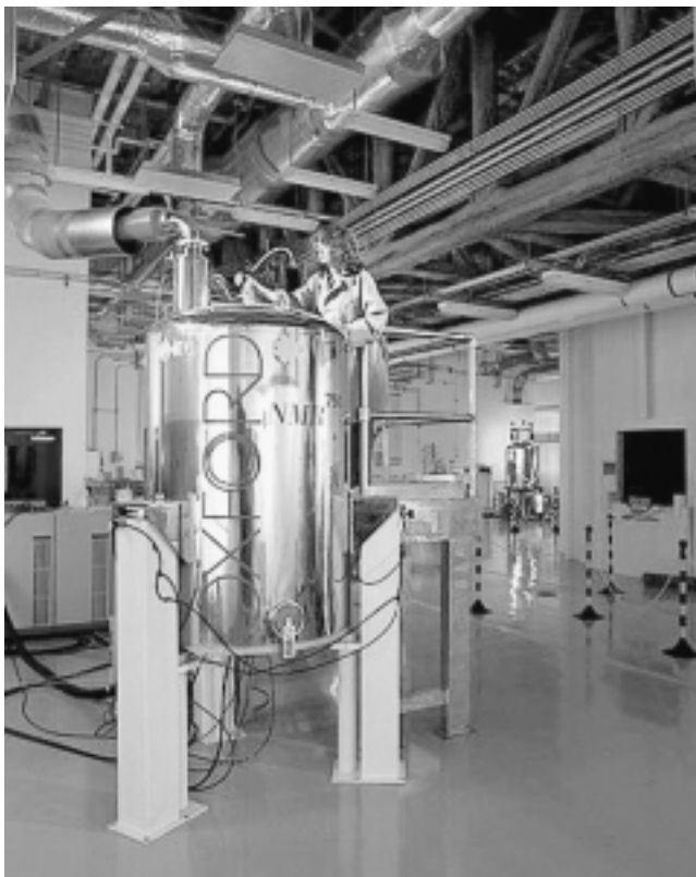
The magnetic characteristics of atomic nuclei play a key role in living processes. These are exploited routinely in nuclear magnetic resonance (NMR) spectroscopy. Here, a spectrometer at the William R. Wiley Environmental Sciences Laboratory in Washington state.
