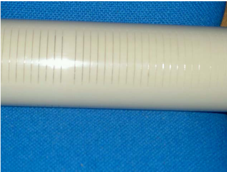
Figure 6.6 Blow up of the tube: Slots of 0.2 mm width are cut in the lower half of the tubes, so water can flow in or out.
