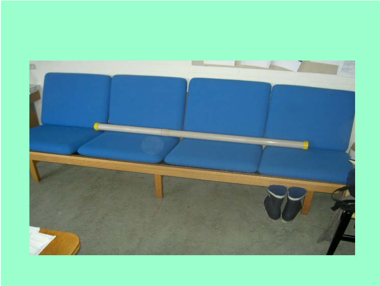
Figure 6.5: Photo of tube in full length. The tube is without slots in the upper half, but it is ventilated at top, so air can go through.
