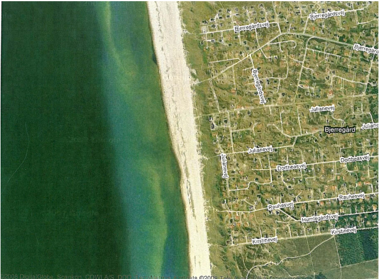
Fig. 11. Aerial photos showing the effect of holes in bars on coastline formation (Digital Globe Scankort, COWI A/S).
