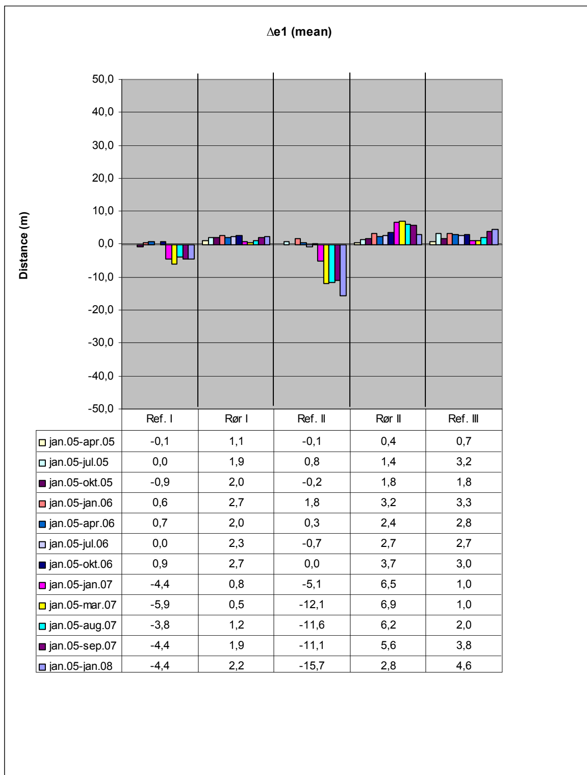
Figure 7.4: Average changes in dune foot position from January 2005 along each individual stretch.
