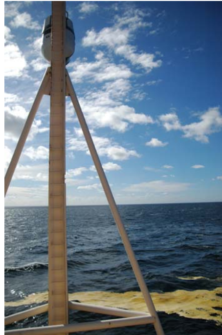
Sensor in the front mast and measuring the oil on the water surface
