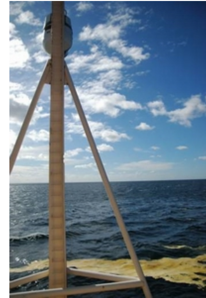
SensorPack mounted in the front mast with oil in front of the vessel
