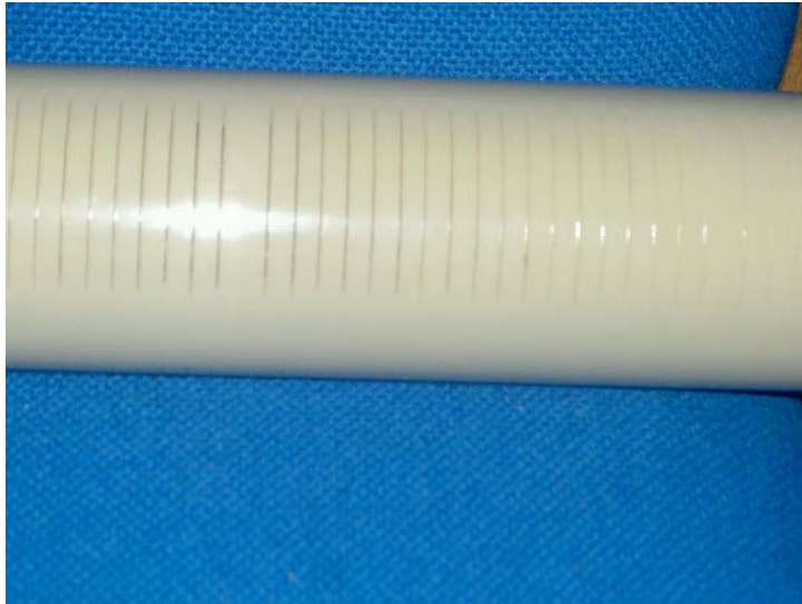
Figure 4.2 Blow up of the tube: Slots of 0.2 mm width are cut in the lower half of the tubes, so water can flow in or out.
