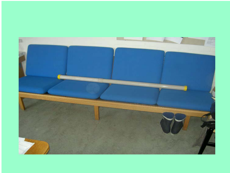
Figure 4.1: Photo of tube in full length, approximately 1.60 m. The tube is without slots in the upper half, but it is ventilated at the top, so air can go through.
