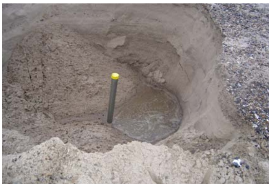
Figure 4.5: It takes 5-10 minutes before the groundwater shows up in the bottom of the hole. This gives an indication how fast you can drain the beach (at least by active pumping).
