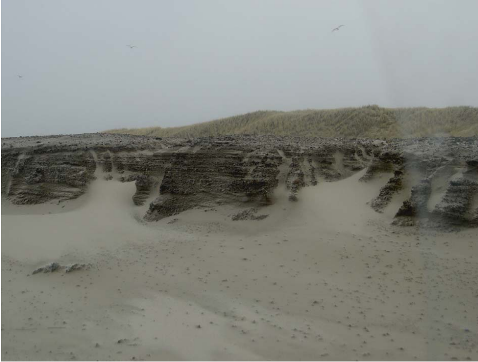
Figure 3.7: The structure of the dune foot varies. Her stratification is observed in the reminiscence of beach nourished sand. Beach nourishment was stopped during the test and only bar nourishment was maintained.
