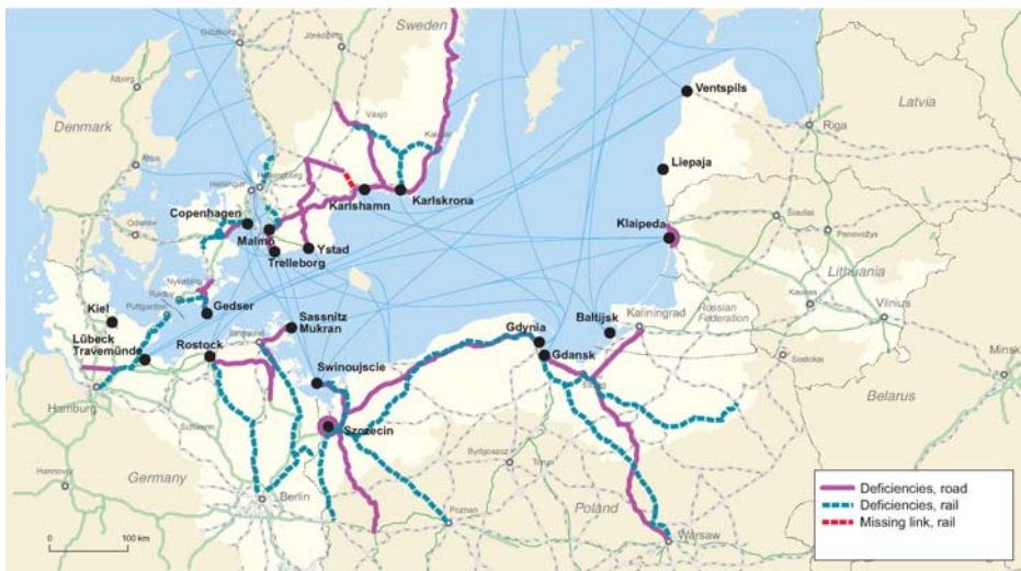
Picture 16: Overview of main shortcomings in the port hinterland connections within the South Baltic Sea area today
