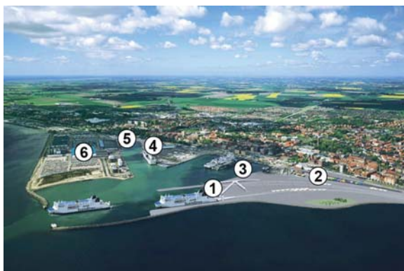
Picture 27: Trelleborg VISION 2005 includes (1) two new railway roro-berths, (2) a new intermodal terminal, (3) a new roro-berth, (4) extension of the check-in area roro terminal 1 (5) a new roro-terminal 2, (6) a new logistics centre
