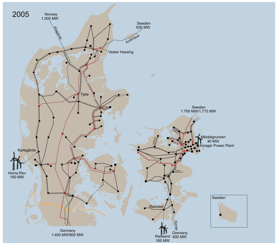
Figure 6.2: Map of the electricity transmission grid in Denmark, showing the location of the three largest Danish offshore wind farms currently in operation and interconnection lines to Norway, Sweden and Germany. Source: Energinet.dk
