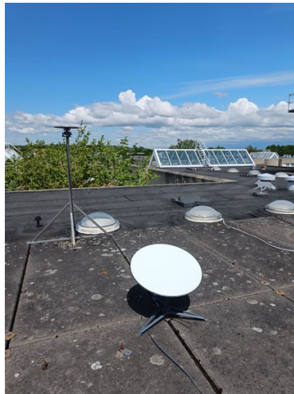
Figure 3. Starlink Residential Generation 1 antenna at test location in Aalborg, Fredrik Bajers Vej 7, Aalborg Øst, facing south.
